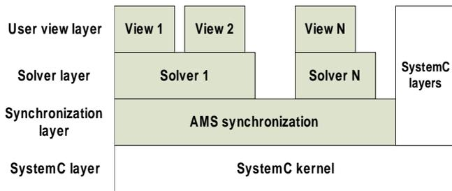
Figure 2. SystemC-AMS layered structure.
