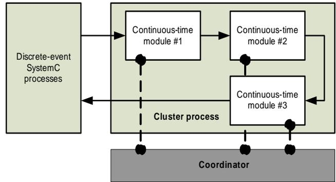
Figure 3. Continuous-time blocks embedded in a dataflow cluster.
